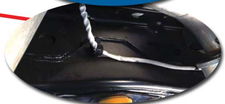
Picture shows 'Yes' inner side plates welded on frame. Old Style
